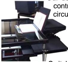
Our design team have created a book handling system with all of the sophisticated pneumatic control of pressure and speed to handle brittle volumes, but with none of the electronic circuitry previously employed. The modular design means that the **GUARDIAN** may be supplied as a simple base unit, easily upgraded with pneumatic book handling facilities at a later date.
